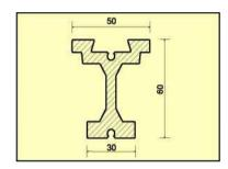
Material: AlMgSi 0.5 Heat treated anodized aluminum
