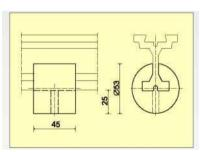
Its function is to close the ends of the curtain tracks. It is made of soft cast VULKOLLAN. It can be rigged using the threaded pin.
