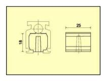
Its function is to close the ends of the curtain tracks. It is made of soft cast VULKOLLAN, and can be rigged using the threaded pin.
