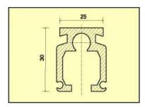
Material: AlMgSi 0.5 Heat treated anodized aluminum
